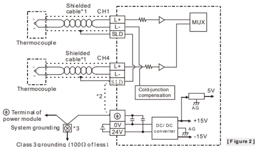
**Note1:** Use only the wires that are supplied with your thermocouple sensor. Tighten PLC terminal screws to a torque of 1.95 kg-cm (1.7 in-lbs).
